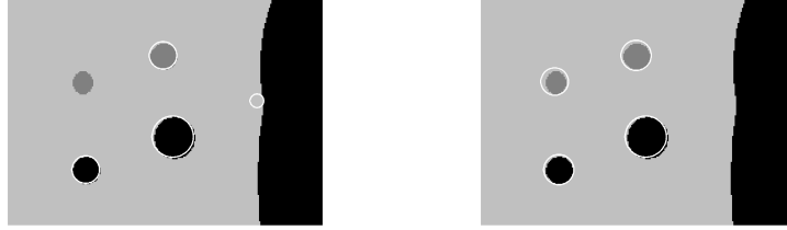
Fig. 3. Shows how edge suppression stops the detection of edges: (left) no suppression and a target is detected on the black edge; (right) suppression is on and all four blobs are detected.
