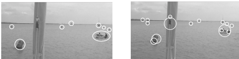
Fig. 1. (left) A typical image, with features of interest manually highlighted in white; (right) what we can achieve with our FRBD.
